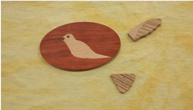
Step#5 Install the inlay collar. Using plate #4 cut out a pocket slightly shallower than your inlay piece. Glue in the inlay piece, Let dry and sand flush.
